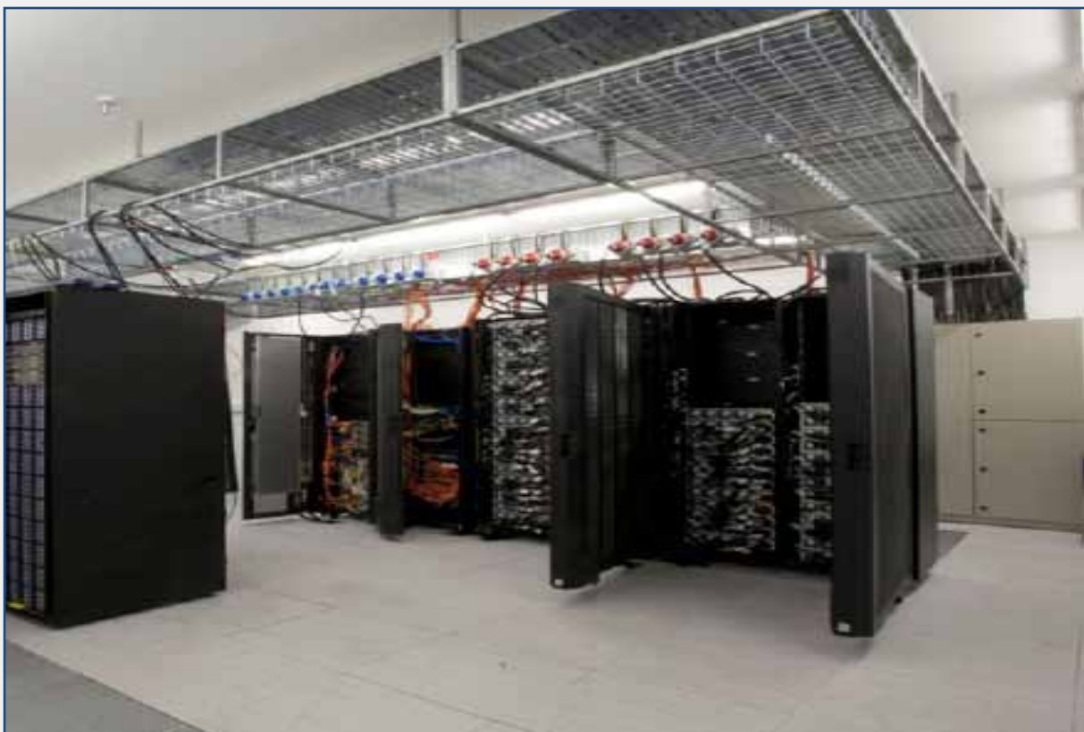
Cy-Tera at the Cyprus Institute: A hybrid machine of peak performance of 30 Tflops
